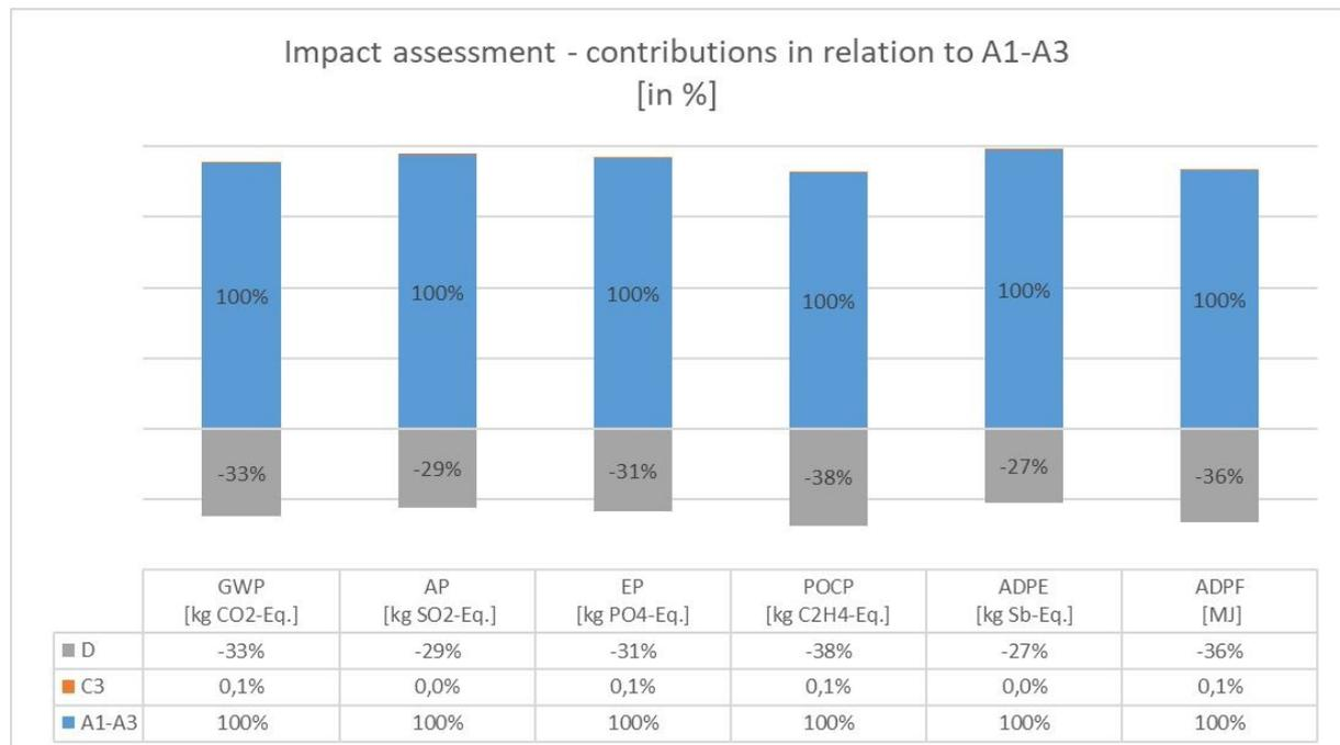
The figure above shows the relative contribution of the production stages (Module A1-A3), waste treatment (Module C3) and the benefits and loads beyond the product system boundary (Module D).
